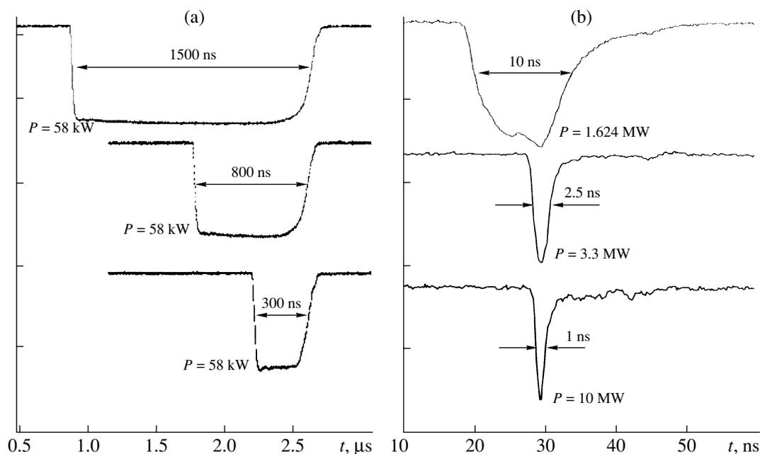
**Fig. 2.** Oscillograms of pulses in the modes for forming (a) microsecond and (b) nanosecond pulses.
