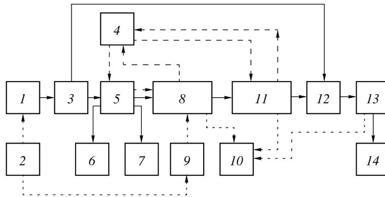
**Fig. 1.** Block diagram of the facility for resonant compression of the microwave energy: (1) microwave transmitter; (2) control unit; (3, 12) waveguide electromechanical switches; (4) gas filling system; (5) phase circulator; (6, 7) circulator loads; (8) first-stage compressor; (9) spark-gap triggering unit; (10) system for signal indicators and parameter measurements; (11) second-stage compressor; (13) coupler; and (14) dummy antenna.
