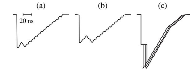
**Fig. 2.** Output pulse envelopes in the cases of (a, b) separate energy extraction through each of the switches, and (c) synchronous energy extraction through the two switches with further summation of the output signals.
